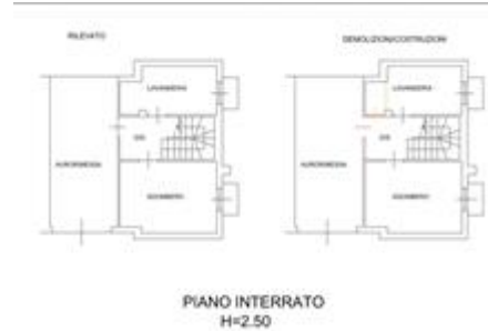
ABUSI PIANO INTERRATO
